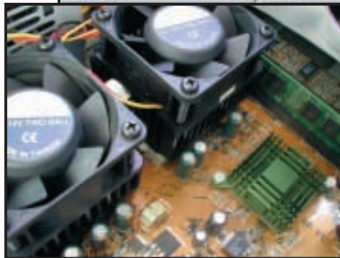
Top: Tucked away in the NT Resource Kit is Perf Meter. This makes it easy to track activity on both processors, plus there's a range of other elements Above: The Abit BP6 motherboard has given many hand-ons experience of multiprocessor systems
